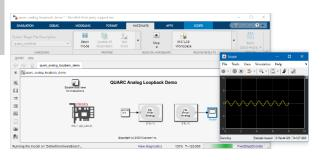
A 1-Hz half-wave rectified sine wave of amplitude 1 should be plotted in real-time. If not, go to the *Troubleshooting* section.
