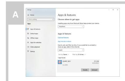
Uninstall any previous version of QUARC that may be present on the computer. Furthermore, if you have the QUBE-SERVO-USB, Q2-USB, or Q8-USB devices, you need to unplug them from the computer before uninstalling the earlier versions of QUARC.
