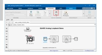
Click on the **Stop** button on the Hardware tab of the Simulink Toolstrip to stop the running model.
